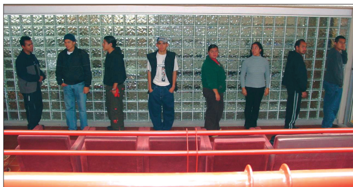
Fig. 2. Students in the detection plane locate the positions of maximum and minimum sound intensity in the interference pattern. The horizontal oscillating rod is not shown.
